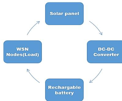
Figure 5. Solar energy harvester model
