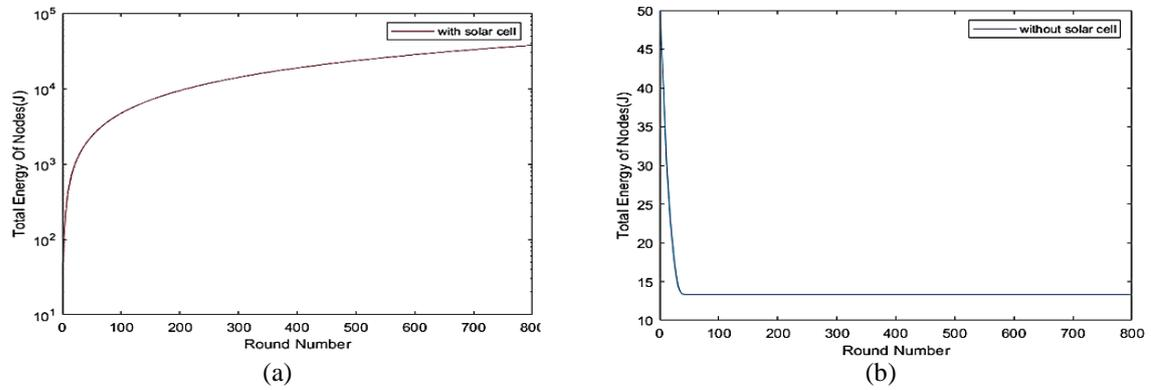
Figure 8. The instantaneous amount of available energy for nodes (a) with energy harvesting and (b) without energy harvesting
